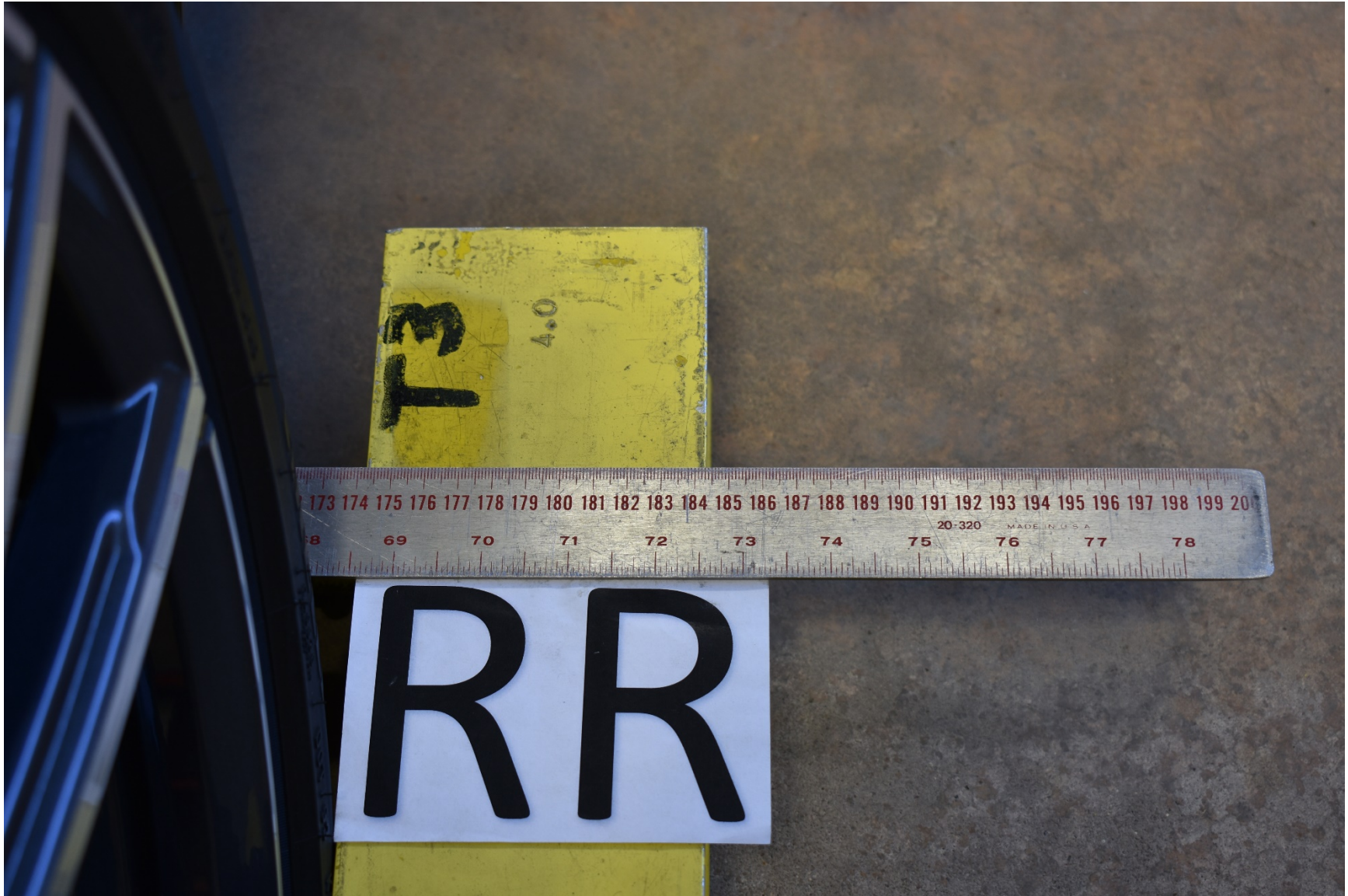
FIGURE 5.19 REAR RIGHT TIRE FRONT MEASUREMENT
